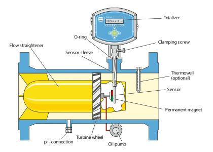
Furthermore, the volume corrector integrated in the TME 400-VCF allows the calculation of the standard volume (VB). In order to do this, the meter measures operating pressure and operating temperature in addition to the operating volume flow. From this, the standard volume flow can be calculated using a suitable equation of state together with the corresponding standard conditions. Then this value is summed up in the standard volume totalizer and stored in the data logger.
